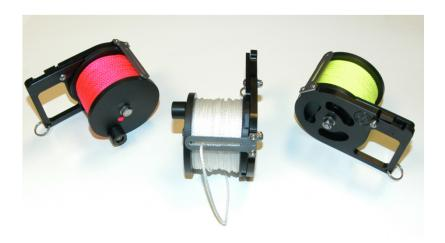
This reel has been designed to offer both ratchet and free run functions. The reel is always set in the ratchet/locked position; to select free running mode, simply depress the spring actioned ratchet pawl with your thumb, which is located just above the main frame handle. This operation can be carried out with same hand that holds the reel. Because of its unique design, the reel is **snag-free** and the tension of the spool run may also be adjusted to suit individual needs.
