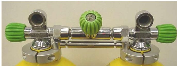
The cylinder lift bar is designed to comfortably lift twinned cylinders on both manifolded and non-manifolded systems. Fitting the lift bar will prevent stress to the manifold itself and o-ring seats. For manifolded tank configurations the lift bar is positioned just below the manifold and therefore takes the full weight of the cylinders. The fully adjustable system allows fitting to twinned 7ltr to 20ltr tank configurations.
